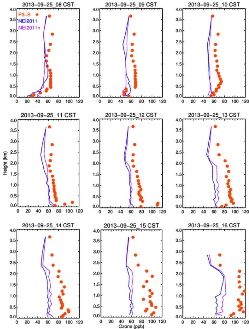
**Figure 3:** Ozone vertical profile – modeled vs. measurements; measurements are aggregated over model grid cells and averaged hourly
